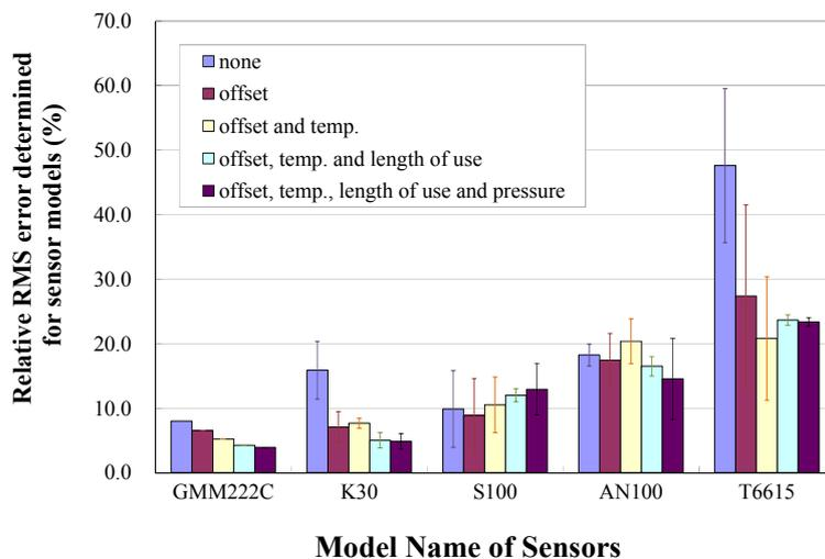
RRMS errors determined for S100 and T6615 were increased with increasing calibration parameters (Table 2). Since the raw outputs of these sensors did not increase linearly with temperature and length of use, the calibration method might not be adequate for these sensor models.
