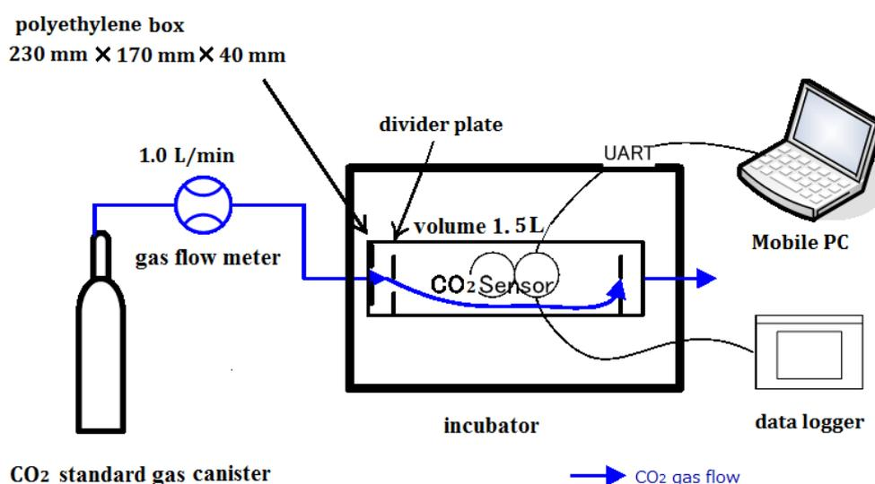
To evaluate the sensors' output dependency on temperature and length of use, CO<sub>2</sub> concentrations of standard CO<sub>2</sub> gases were measured with the individual sensors for different temperatures and durations. Electrical power was supplied to the individual sensors 30 min before the start of the experiment. The standard CO<sub>2</sub> gas was sent to the sensor box at a flow rate of 1 L/min.
